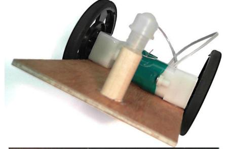
Adjust the length of the dowel so that the base is level.
